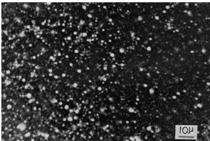
Fig. 10. Phase contrast micrograph of SBR-B (25% styrene content, without block)-GP polystyrene resin blend (70/30 weight ratio, after remilling), prepared by mill blend. Heat treatment: 150°C \times 5 hr. Asker C hardness: 48.
